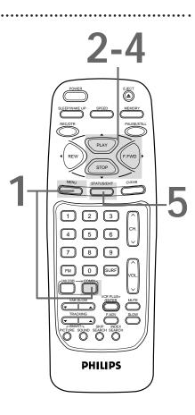
Press the PLAY/ $\blacktriangle$  button or the STOP/ $\lor$  button to select SET CLOCK. Then, press the F.FWD/ $\triangleright$  button.
